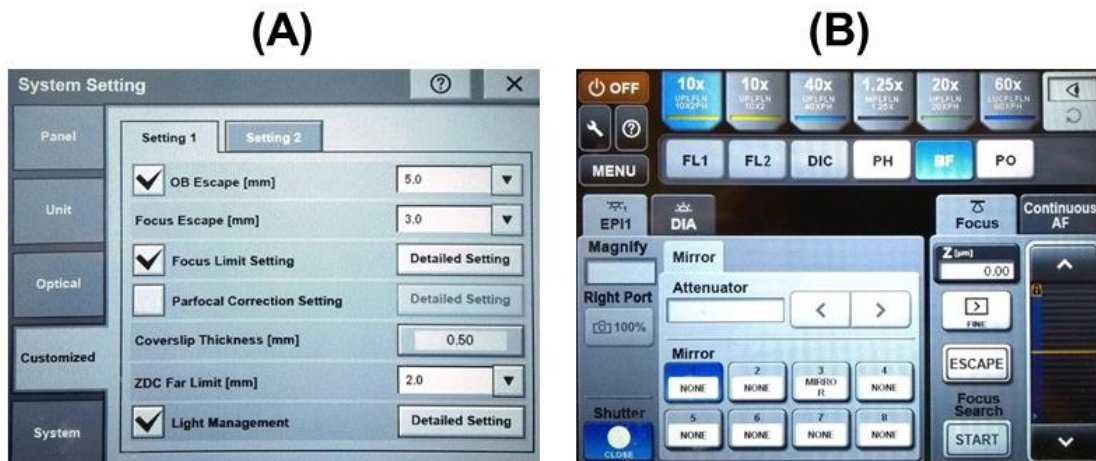
Figure C.2 Focus Settings on the touch pad of the IX83 microscope. (A) In order to activate the Z drift compensating IX3-ZDC module, Focus Limit Setting needed to be checked. (B) The main control panel showing a yellow line at a certain Z position. This indicates the ZDC has been activated and ready to be controlled by the GUI.
