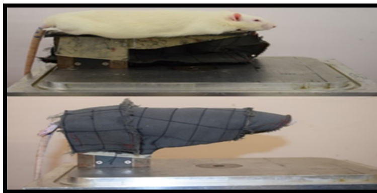
Figure 2.2: Anesthetized rat strapped and secured on the surfboard before mounting onto the test chamber. Strapping the animal prevents the head or body motion during the propagation of the shock wave.
