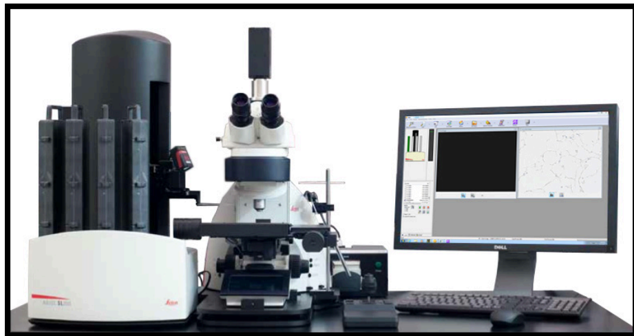
Figure 2.5: Leica Aperio Versa 200 fully automatic digital slide scanner with fluorescent microscope used in the present study to digitize the images of various brain regions and analyze the fluorescence intensities of NOX 1 and NOX2 proteins.
