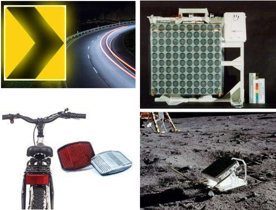
Figure 1.4 Examples of common retroreflectors in road signs and bicycles (left) and Lunar Laser Ranging Retroreflector on the moon (right)
