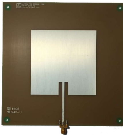
Figure 1.7 Example of inset-fed patch antenna with a microstrip feed line.
