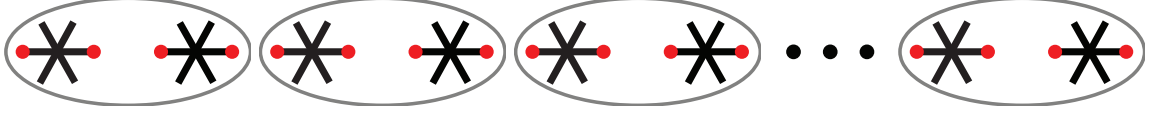
Figure 4.3 The 1D spinner system with the open edge. Grey line demonstrated unit cells.
