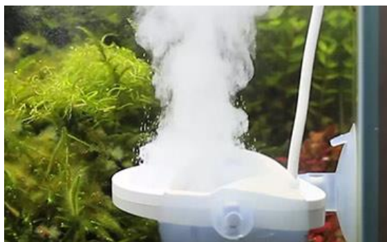
Figure 3.6 Electrolysis bubble generation in fish tank.
