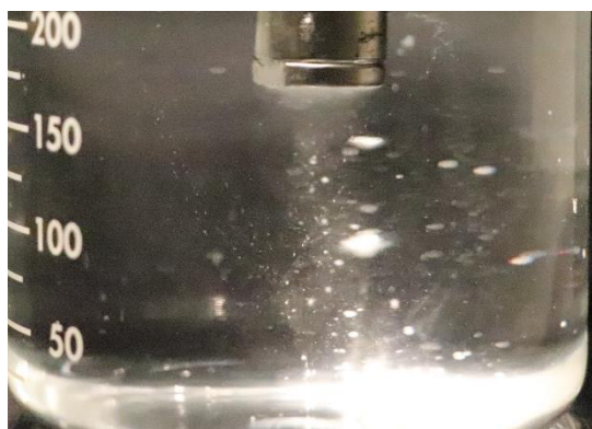
Figure 3.5 Bubble cavitation under ultrasound probe.
