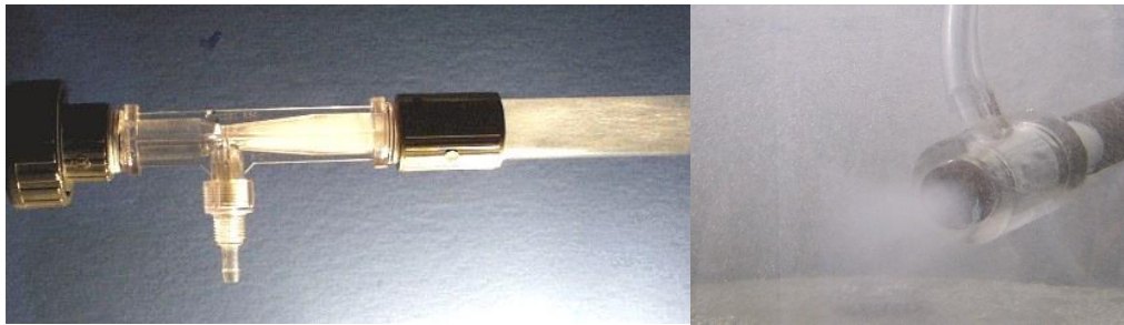
Figure 3.4 Venturi type nano-bubble generator.
