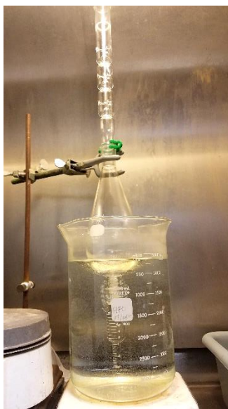
Figure 4.3 Kuderna-Danish concentration sample preparation for GC/MS.
