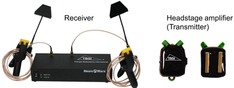
Figure 2.8 64-channel wireless recording system (Triangle BioSystems International).
