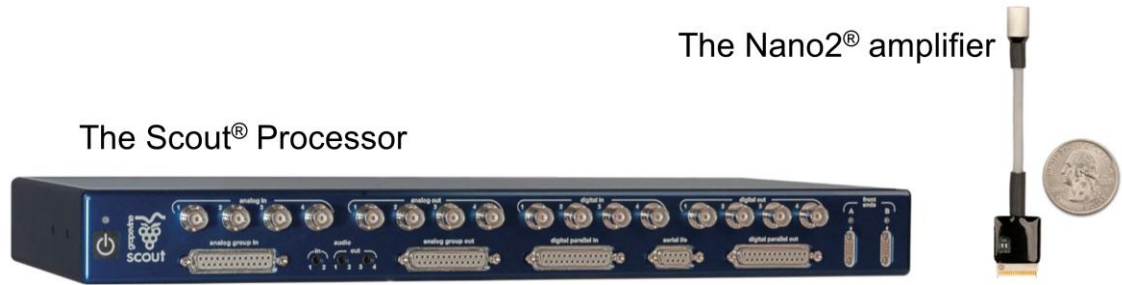
Figure 2.9 Tethered front-end amplifier (RippleNeuro, UT).
