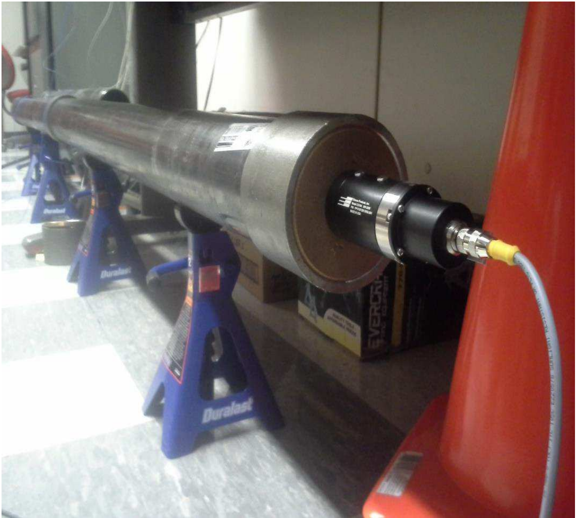
Figure 3.2 The transmit transducer mounted along the drill string testbed axis.
