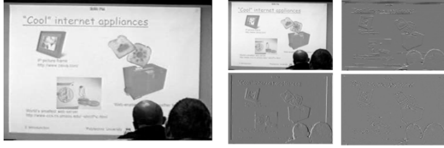
Figure 3.6 Wavelet decomposition, when wavelet transform is applied on image, the image is decomposed into various bands as seen (original image, LL, LH, HL and HH bands).
