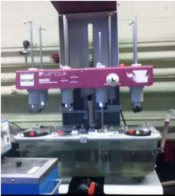
Figure 3.5. Distek 2100B Dissolution System used in this work to support the Minivessel.
