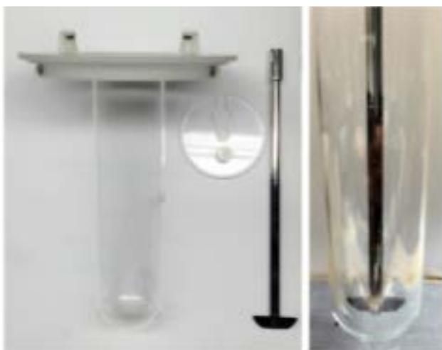
Figure 3.3 (b) mounting plate to adapt minivessel to standard opening for USP2 vessel in typical dissolutin testing system.
