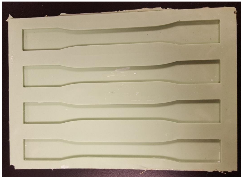
Figure 4.3 Dog bone mold utilized for tensile testing of polymer samples.
