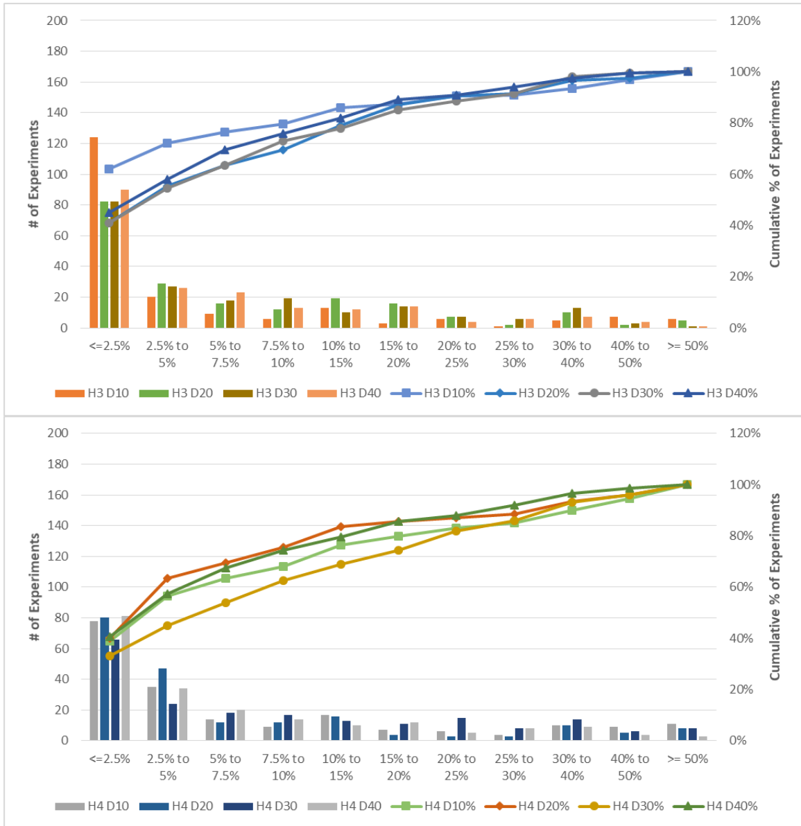
Figure 4.12 The performance analysis illustrates H3 is outperforming with a small searching band of 10 while H4 dominates on delta of 40 instead, compared with optimal solution in MILP Model (4.3).
