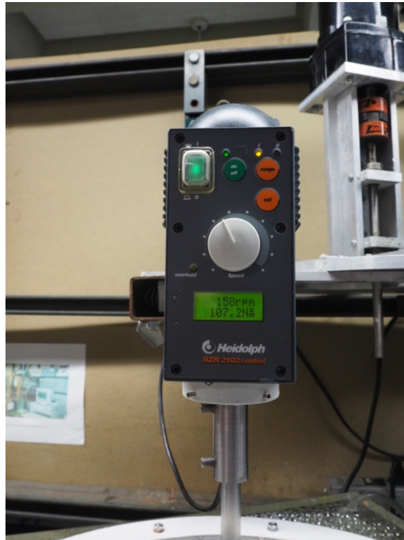
Figure 3.6 100 W motor with accurate internal torque meter (Heidolph RZR 2102 Control).
