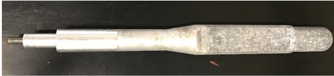
Figure 3.2 Single beavertail baffle used for partial baffling.
