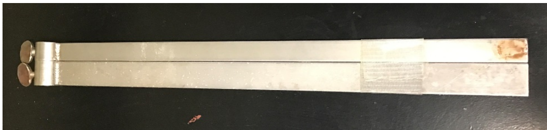
Figure 3.3 Flat baffle used for full baffling. Four such baffle were used in the fully baffled configuration.
