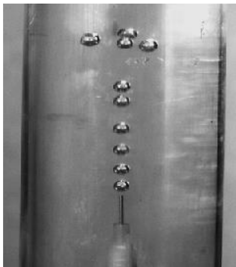
Figure 3.10 Bubbles generated by 23 Gauge needle after cutting.
