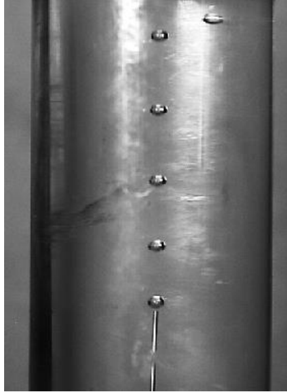
Figure 3.9 Continuous stream of individual separated bubbles generated by 23 Gauge needle.
