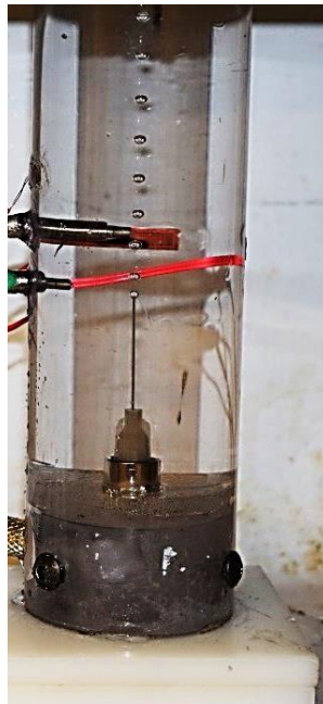
Figure 3.11 Generation of bubbles in 50% glycerol-water solution using 27G needle.
