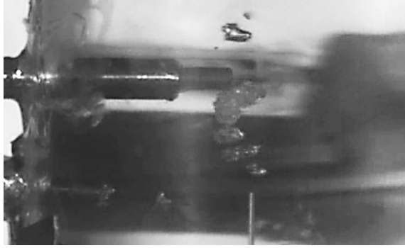
Figure 4.7 Air bubbles in 50% glycerol-water solution- 11.6 ms after the trigger.
