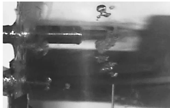
Figure 4.5 Air bubbles in 50% glycerol-water solution- 10.2 ms after the trigger.
