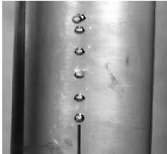
Figure 3.8 Bubbles generated by 22 Gauge needle.
