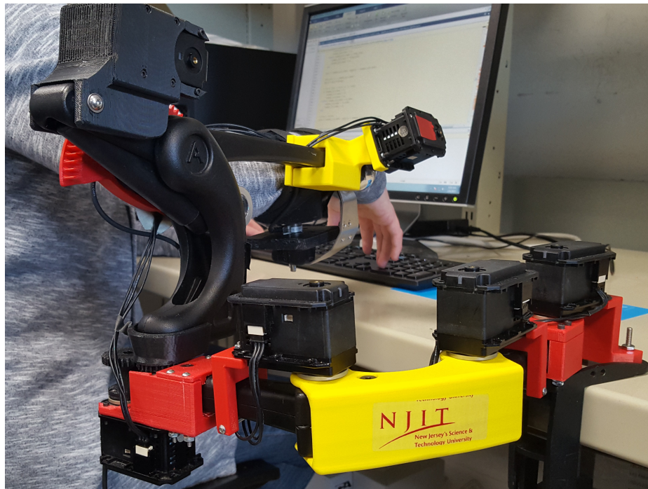
Figure 6.3 The phase 2 prototype of the multi-DOF Armon Edero retrofit with motors and force sensor to operate under admittance control in 3 DOFs.
