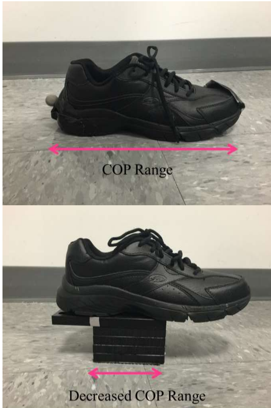
Figure 2.3 The above Figure shows the reduction COP range of shoe with Blocks compared to Regular shoe.
