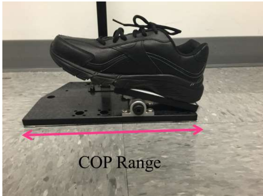
Figure 2.4 Shoe with a pivot and trekking pole to study the ability of the hands to compensate for the confining COP in A/P plane.
