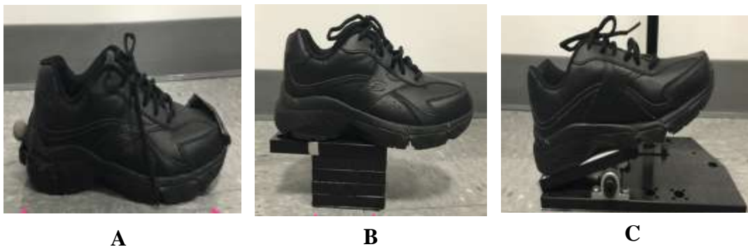
Figure 2.1 A: The commercial running shoes used in Aims 2-4. B: Blocks shoes with the range of COP limited. C: Pivots shoes, Pivots located below the expected COP.
