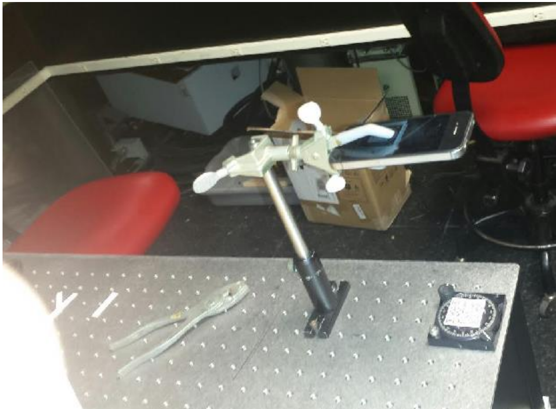
Figure 2.4 The angle test set-up as well as the fluorescent ambient light test set-up.
