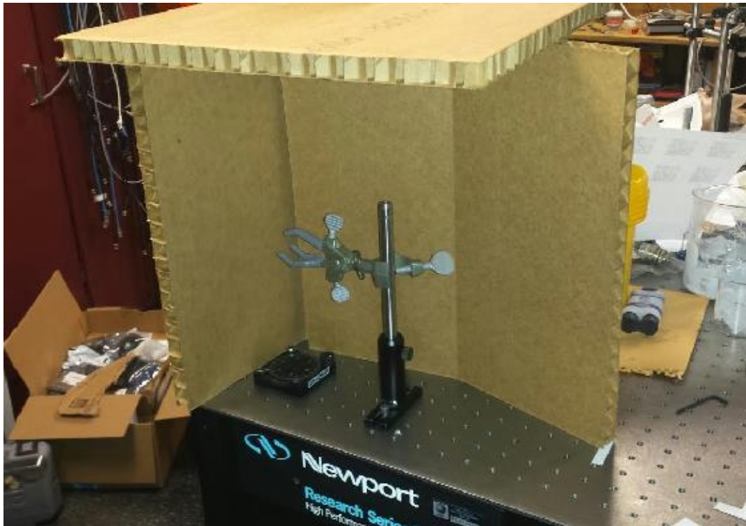
Figure 2.6 The low light level ambient light test set up.
