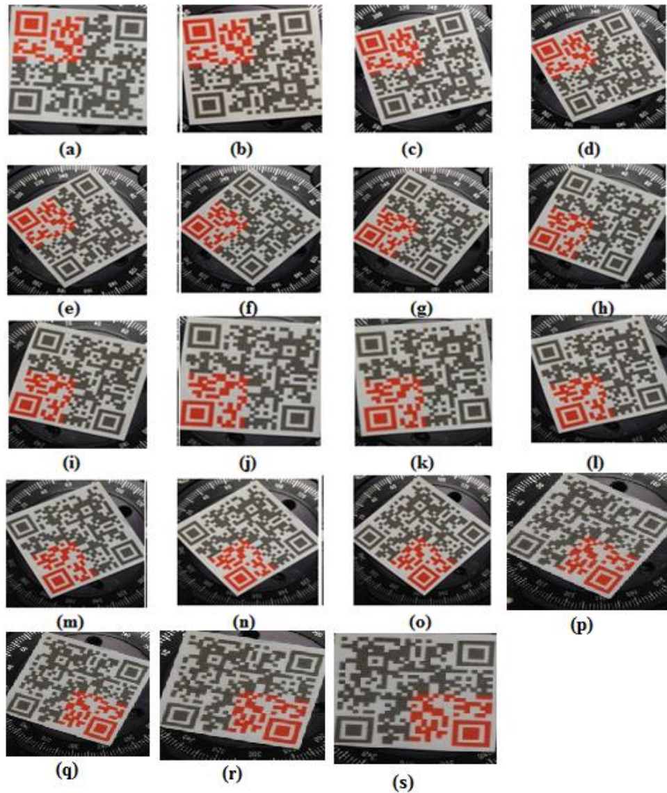
Figure 3.6 The angle test done with a sample in red phase under fluorescent light. (a) 0 degrees (b) 10 degrees (c) 20 degrees (d) 30 degrees (e) 40 degrees (f) 50 degrees (g) 60 degrees (h) 70 degrees (i) 80 degrees (j) 90 degrees (k) 100 degrees (l) 110 degrees (m) 120 degrees (n) 130 degrees (o) 140 degrees (p) 150 degrees (q) 160 degrees (r) 170 degrees (s) 180 degrees.
