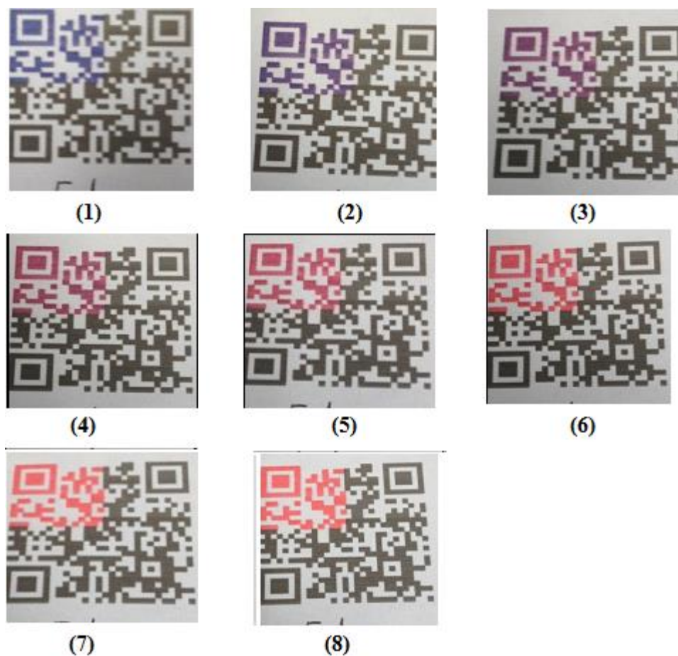
Figure 3.12 One of the chloroform based ink samples through different stages of its transition. Starting from the top left going right are the pictures at (1) 30 degrees Celsius (2) 60 degrees Celsius (3) 65 degrees Celsius (4) 70 degrees Celsius (5) 75 degrees Celsius (6) 80 degrees Celsius (7) 85 degrees Celsius (8) 90 degrees Celsius. You can clearly see the purple phase that is between the blue and the red phase take place from (2) and (6), spanning around 20 degrees Celsius.
