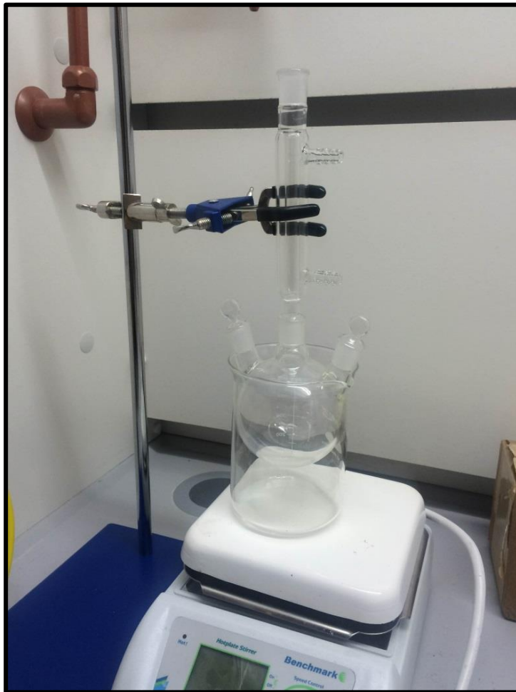
Figure 4.3 Experimental Set up for CNT oxidation that incorporates an in-house reflux condenser built in the chemical hood in the lab.
