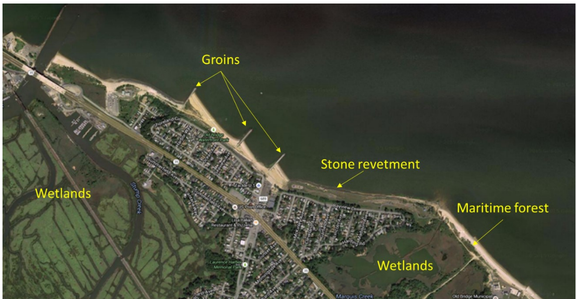
Figure 3.3 Laurence Harbor aerial (500ft), showing location of groins, seawall revetment, beach, maritime forest and wetlands.
