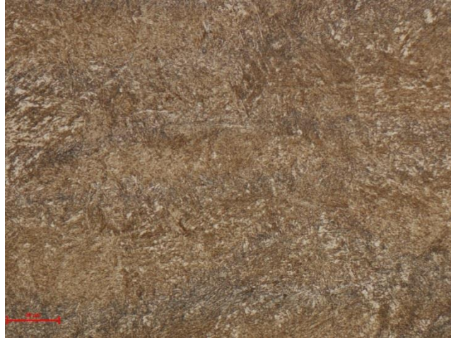
Figure 3.5 DMLS 4140 steel. The scale bar represents 20 microns.
