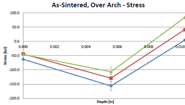
Figure 7.1 Residual stress results - courtesy of American Stress Technologies for the as-sintered condition over the arch.
