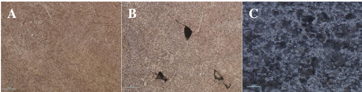
Figure 9.1 Etched Microstructures of 4340 samples, Low porosity parameter (A), under exposed parameters (B), and wrought (C) the scale bar represents 20 microns. Source: [76].
