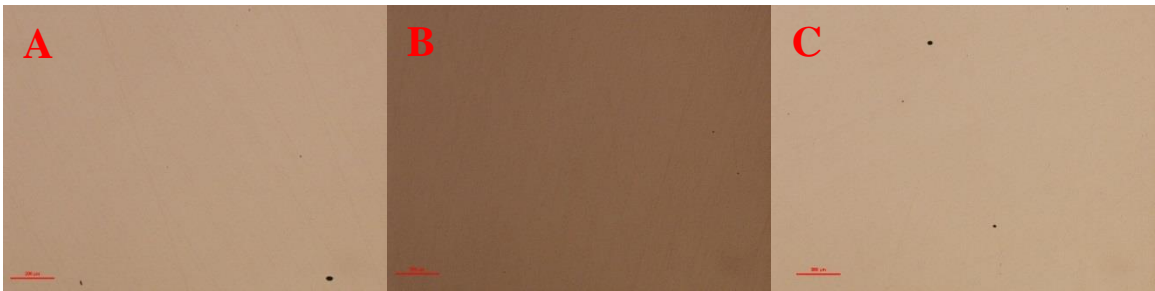
Figure 2.10 50x unetched image of the microstructure of the powder (A) -325Mesh+16 \mu\text{m} , (B) -325Mesh+22 \mu\text{m} , and (C) -270Mesh+22 \mu\text{m} at 185W and 725mm/sec. The scale bar represents 200 \mu\text{m} .
