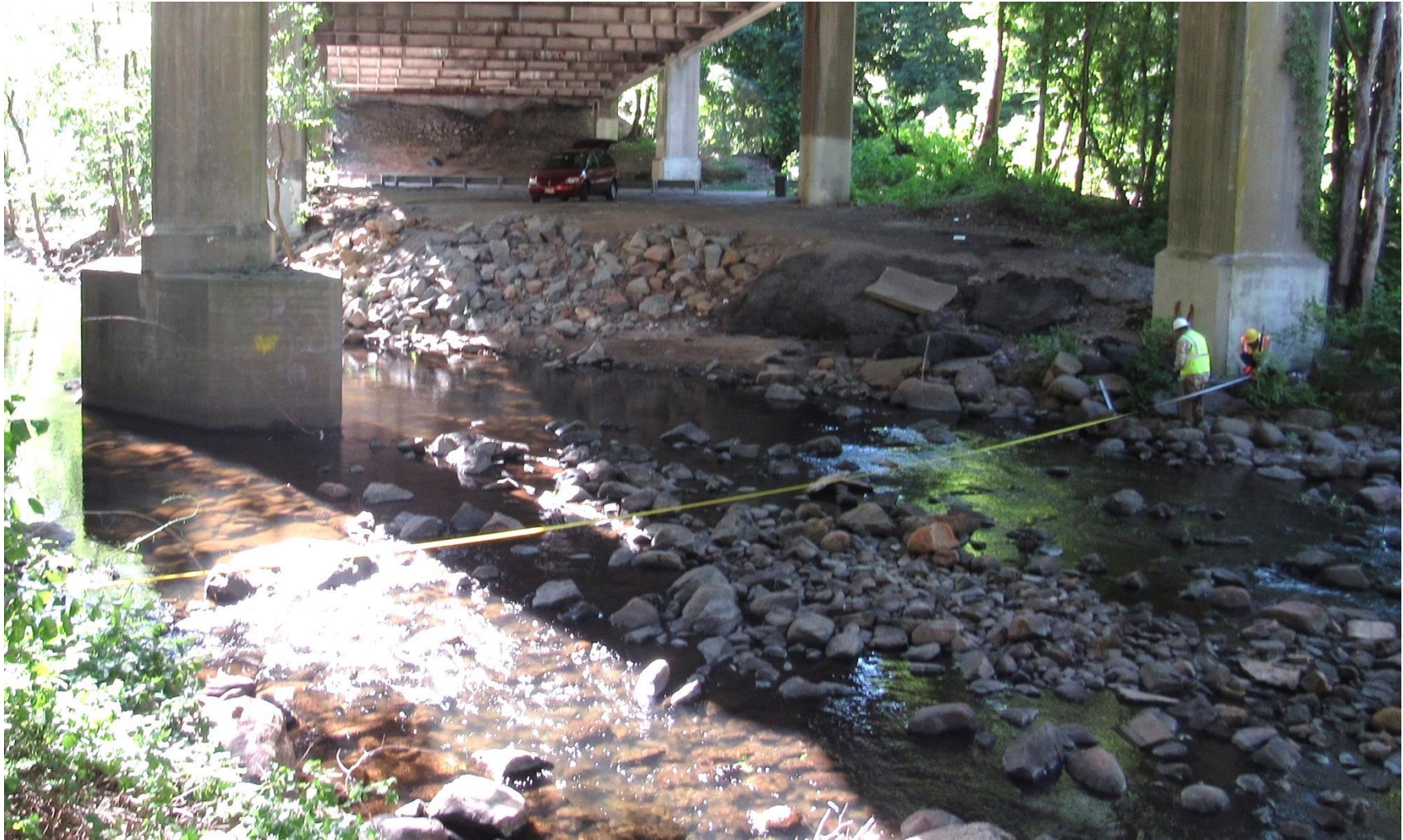
Figure 3.4 Wolman Pebble Count section installation, bridge # 1405-156.
