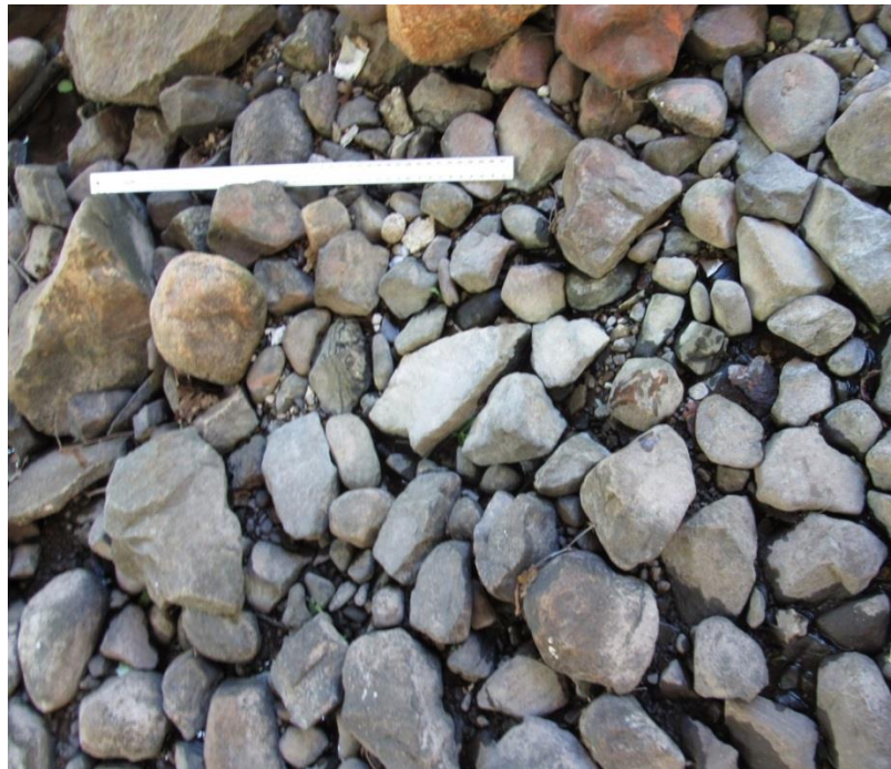
Figure 1.2 Comparison of sand and gravel sediments with extremely coarse particle (ECP), including cobbles and boulders.
