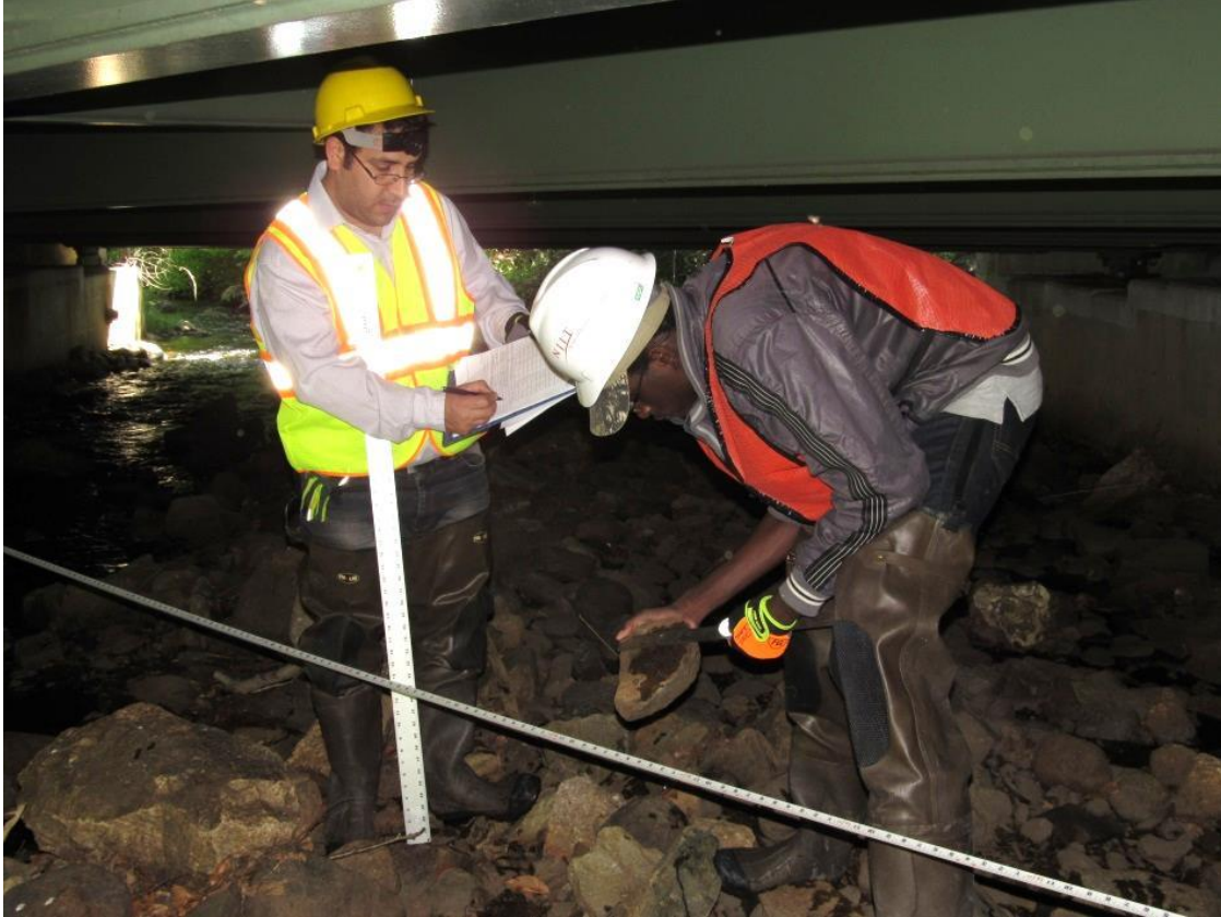
Figure 3.3 Wolman Pebble Count particle selection and measurement.
