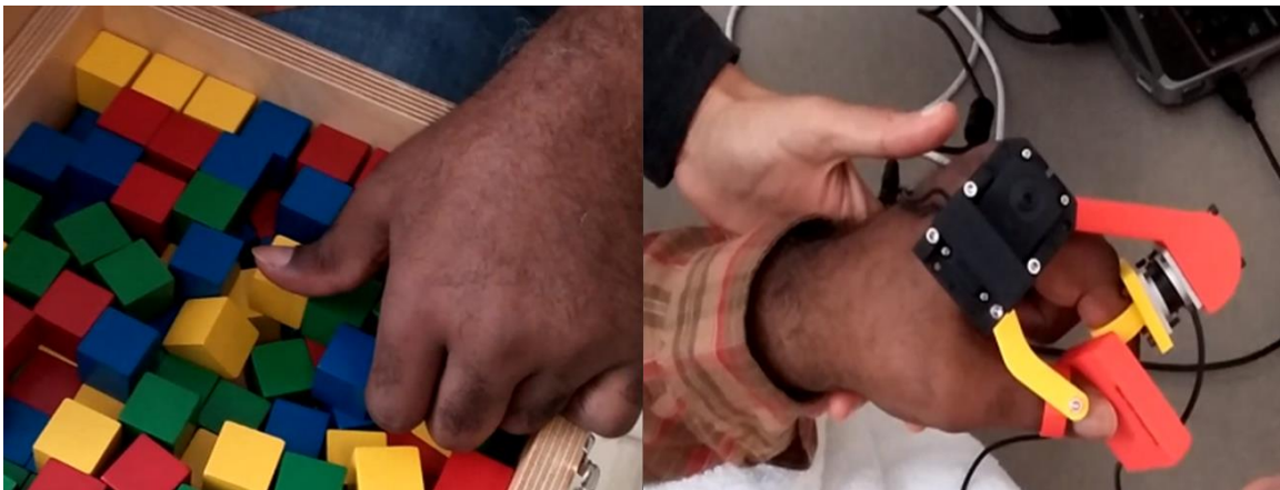
Figure 8.4 Left) Subject CN unable to grasp cube during Box and Blocks Test. Right) Subject CN with modular gripper assisting pinch movements and pinching block.
