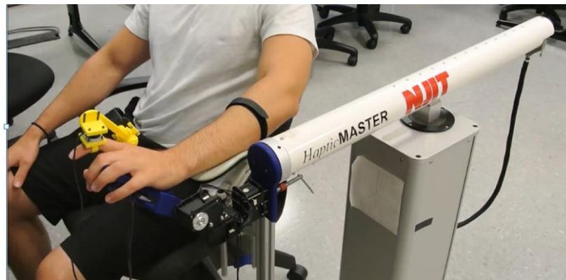
Figure 4.1 NJIT HandsOn System complete with 3 proximal DOF at the shoulder, 3 DOF at the wrist, and 1 DOF for pinch.
