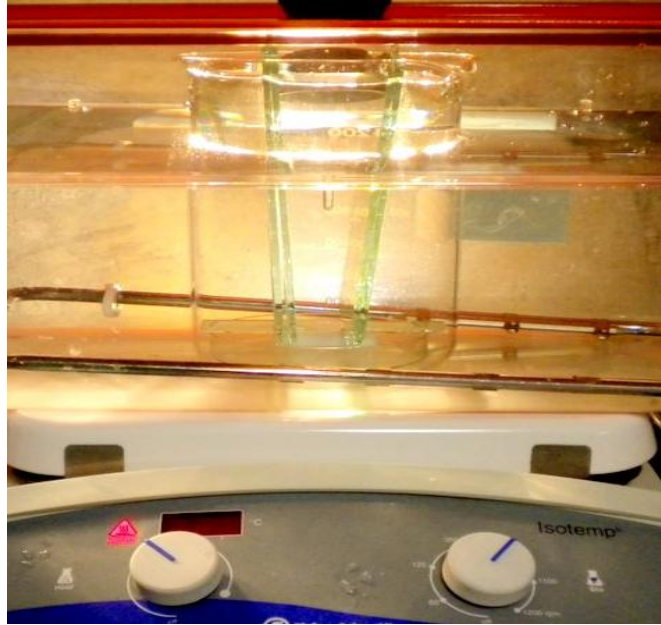
Figure 2.3 Chemical bath deposition (CBD) setup.
