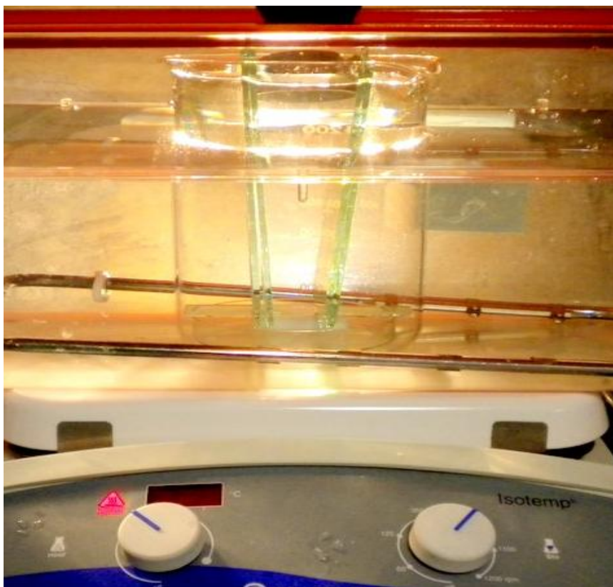
Figure 3.3 Chemical bath deposition (CBD) setup.
