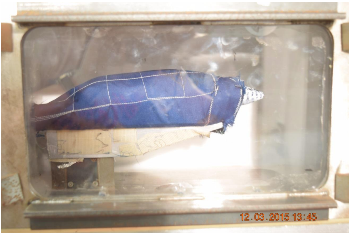
Figure 5.2 RTD inside the shock tube with a harness.
