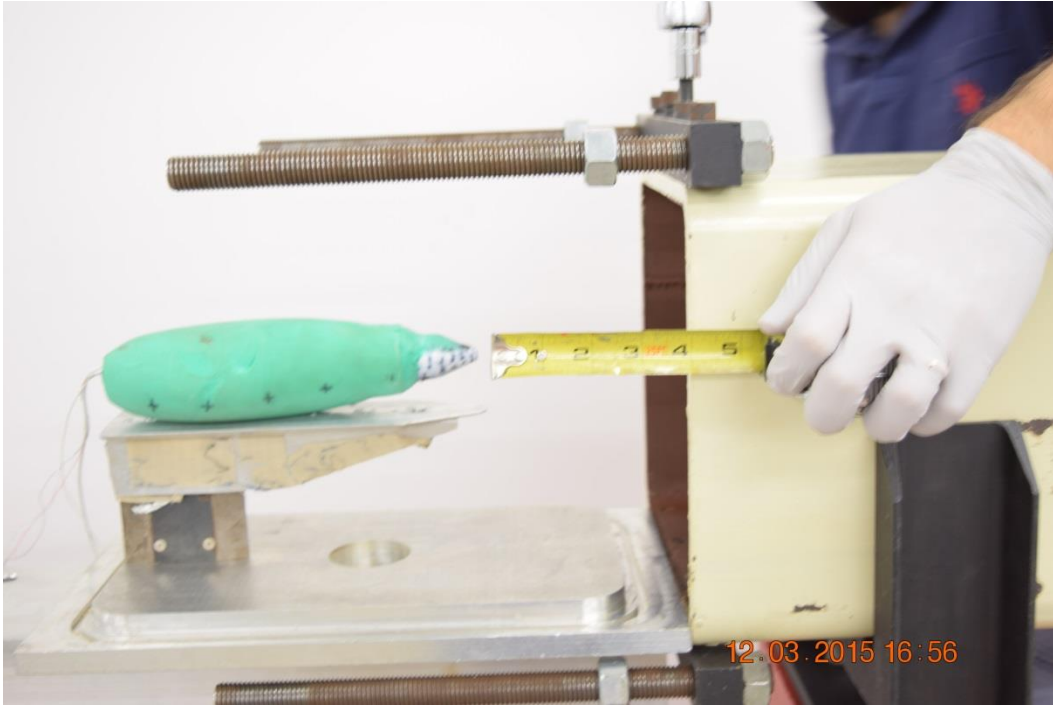
Figure 5.4 RTD unstrapped outside shock tube barrel.
