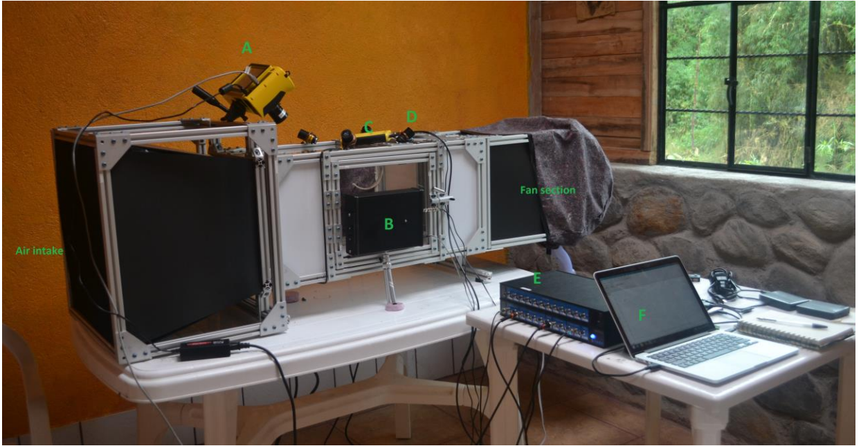
Figure 2.1 Experimental setup. (A) High-speed camera, (B) Speaker, (C) Microphone, (D) Infrared lights, (E) 1401 data acquisition system, and (F) Computer.
