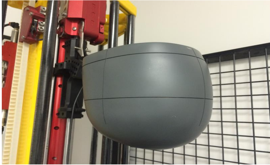
Figure 3.6 The impactor with head shape was used in this experiment to mimic the blunt impact to the head model. The weight of the impactor is 10 pounds, which is close to the weight of a human head.
