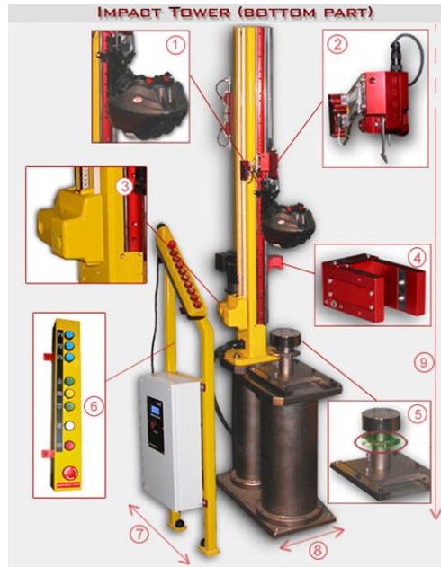
Figure 3.5 The basic structure of the impact machine includes 6 major features: Drop follower (1); Soft release system (2); Electronic encoder measuring system (3); Velocimeter, which can be regarded as the time gate used for speed measuring (4); Quick and easy interchangeable anvils (5) and remote control (6), which usually was used to input different value of the height, and start or stop the test during the experiment.
