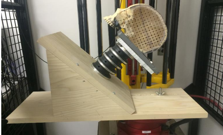
Figure 3.7 The shelf with 45 degree angle was used for the impact test of forehead position.
