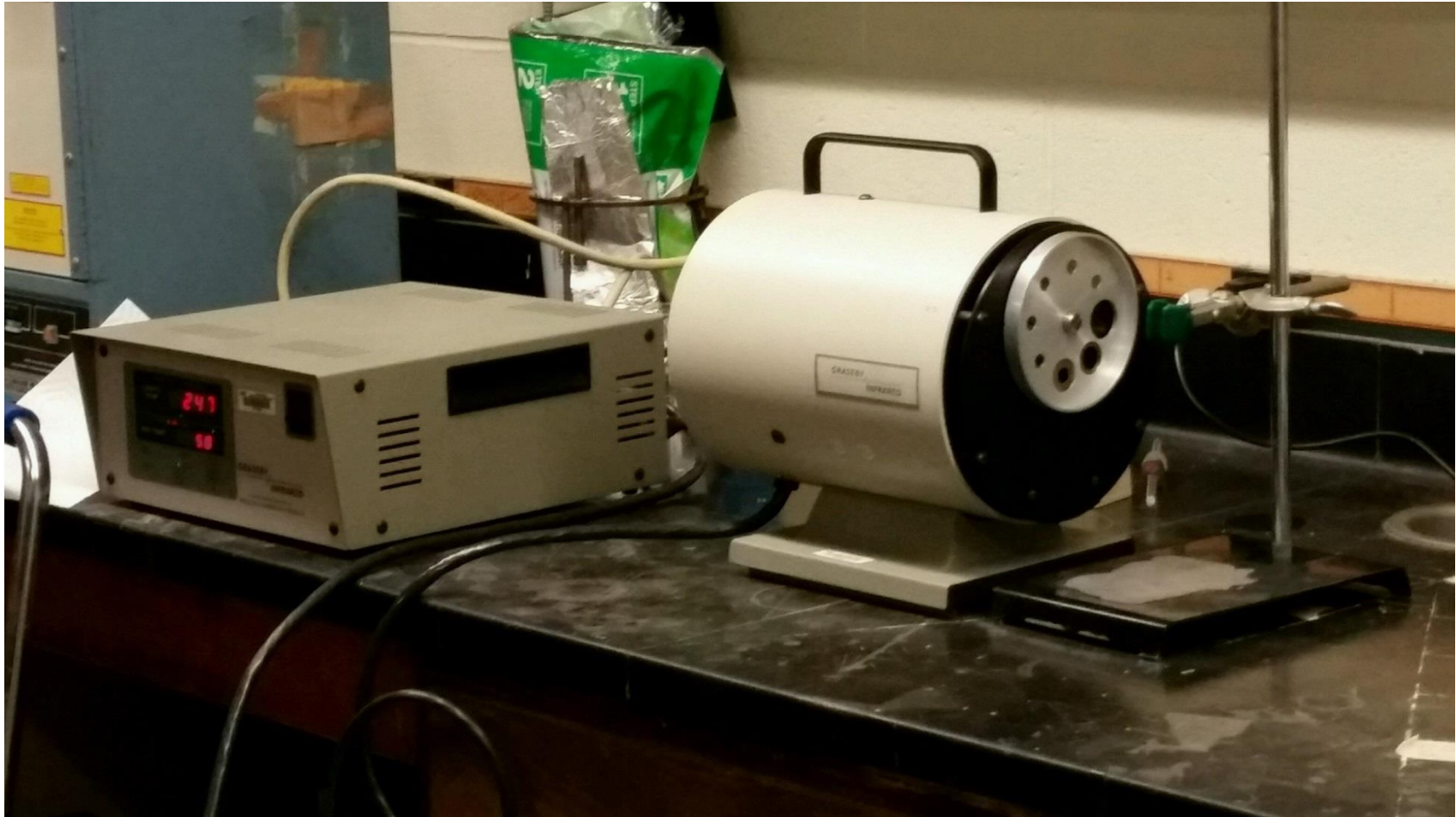
Figure 5.1 Shows the experimental setup with the IR -563 Blackbody Source and clamping apparatus.
