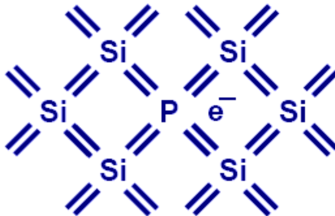
Figure 3.1 Shows the impurity, phosphorous, added to crystalline silicon along the lattice. The addition of phosphorous and its subsequent substitution of a silicon atom in the silicon lattice makes the silicon n-type. Source: [10].
