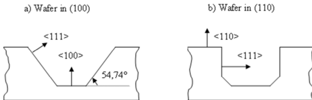
Figure 1.1 The difference between etching rates of (100) and (110) orientation.
