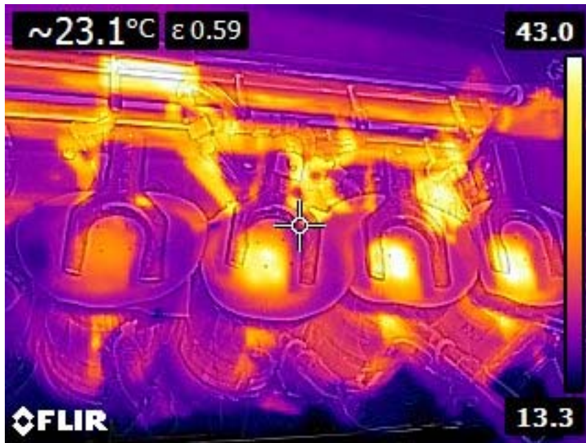
Figure 4.4 Thermal image of cells 1-4* during the diffusion run (top view). * Cell 4 is the left cell and it is the nonheated control.
