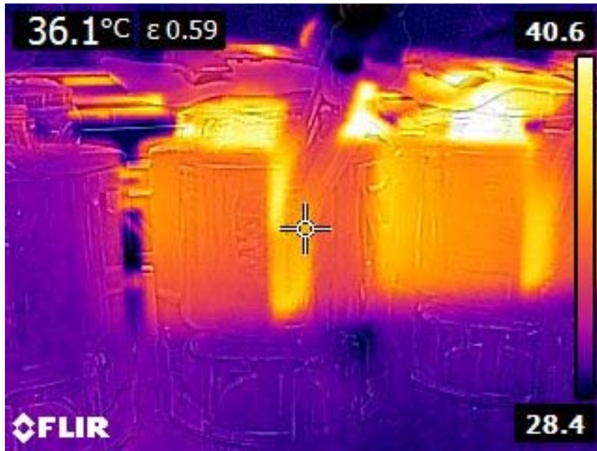
Figure 4.3 Thermal image of cells 3 and 4* during the diffusion run (side view). * Cell 4 is the left cell and it is the nonheated control.
