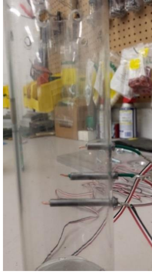
Figure 2.9 Dummy sensors placed inside the cylinder oriented at different lengths.
