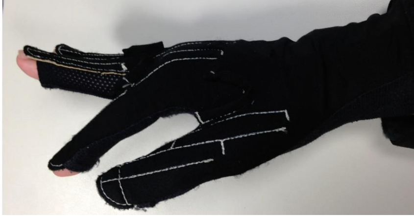
Figure 2.4 CyberGlove. Instrumented gloves (Immersion Co., San Jose, CA) were used to track finger movements.
