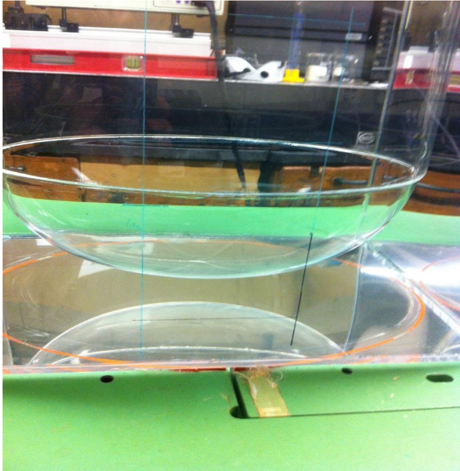
Figure 2.9 Details of the elliptical tank bottom.
