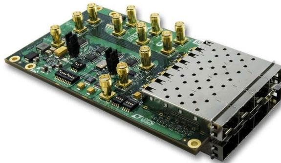
**Figure 4.2** The SFP HSMC Card.
