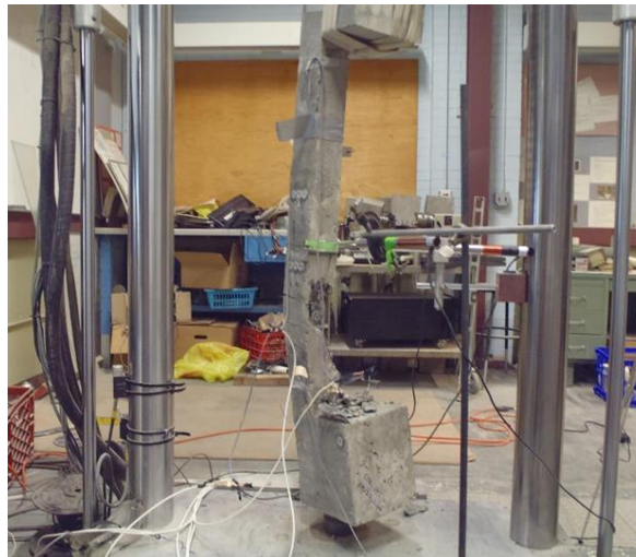
Column C5 at failure
