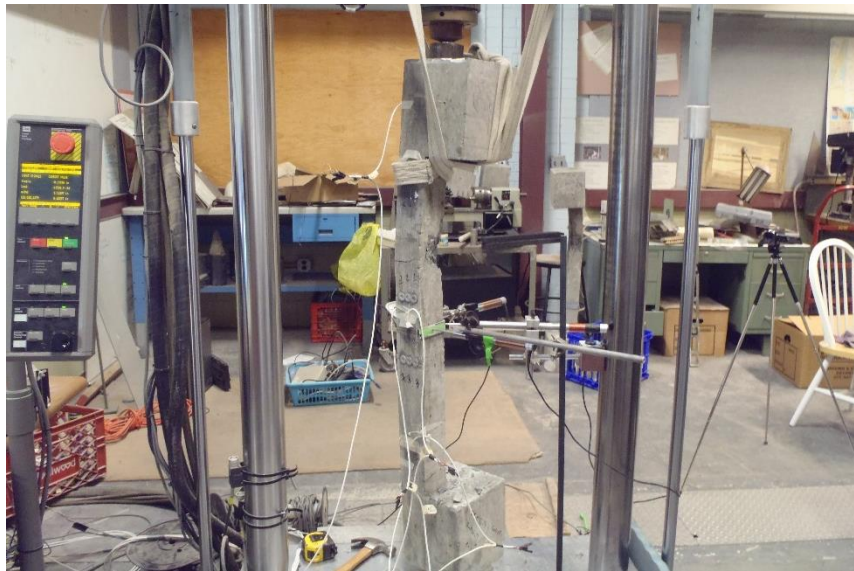
Column C6 at failure
