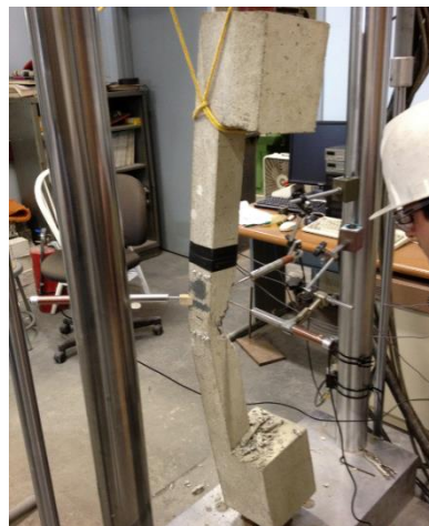
Column C1 at failure
