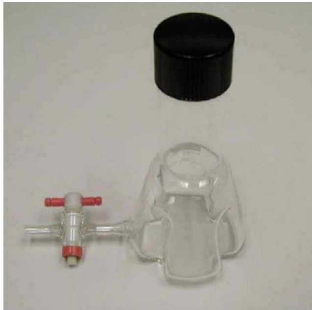
Figure 2.1 Photograph of a baffled trypsinizing flask.
