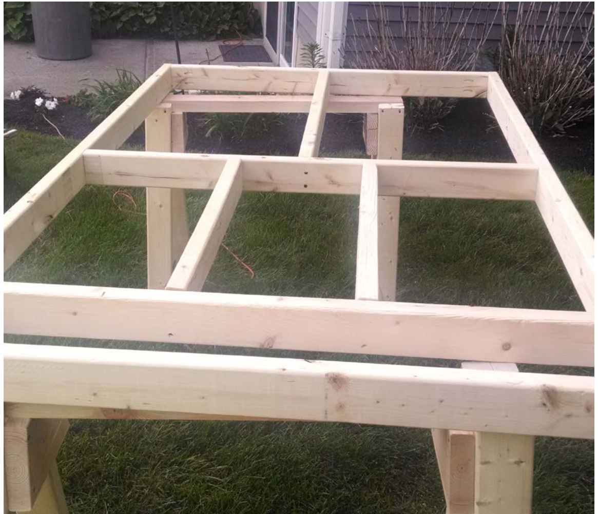
Figure 2.1 Upper deck of Haploscope. Shown here without particle board covering. Saw horses were used only for assembly.
