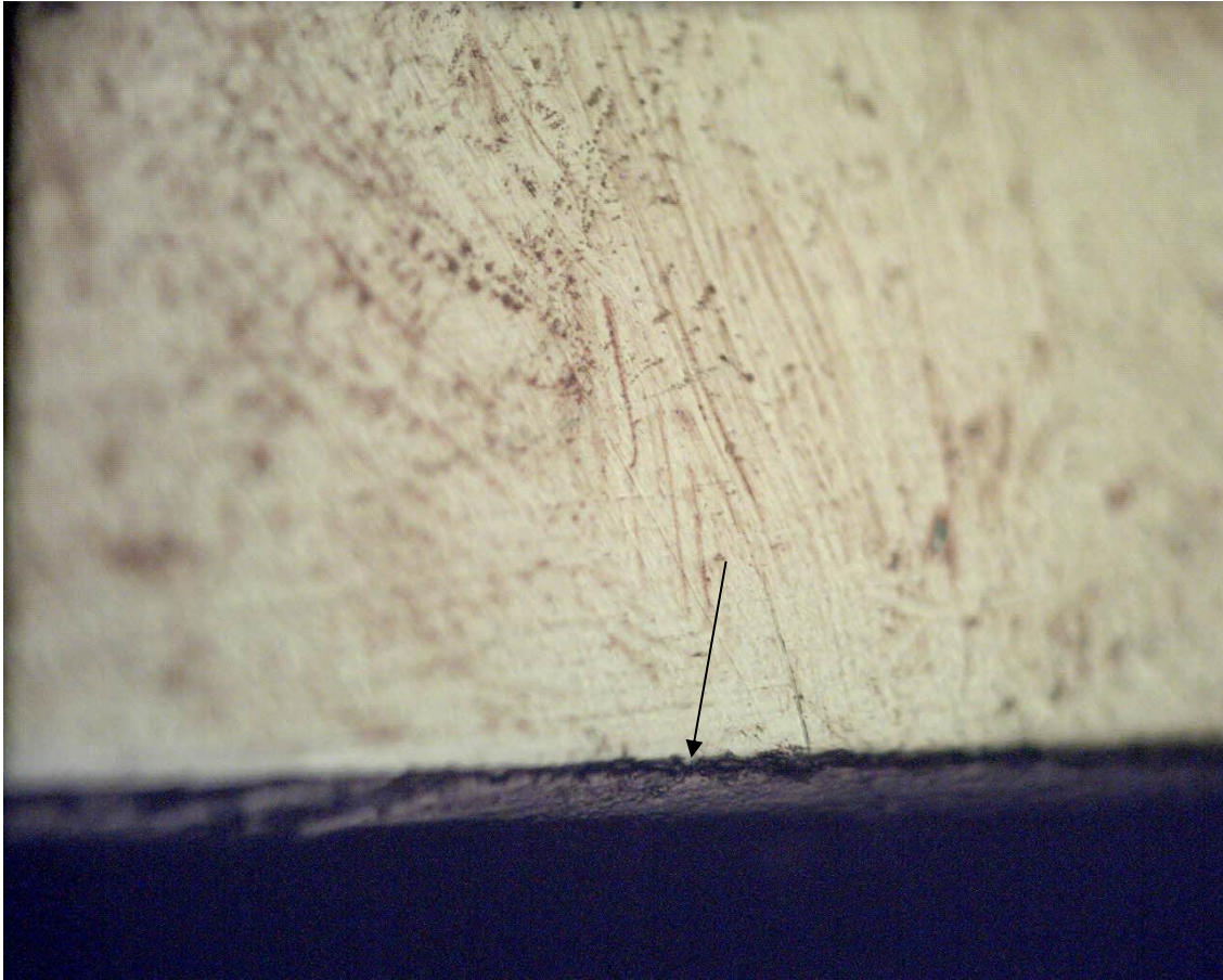
Figure 3.3 Optical image of cross-sectioned Ti-6Al-4V PEO treated sample,100x.
