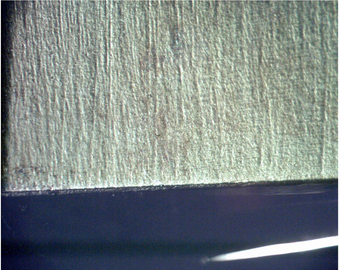
Figure 3.2 Optical image of cross-sectioned Ti-6Al-4V PEO treated sample, 50x.
