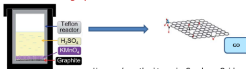
Hummer's method to make Graphene Oxide
