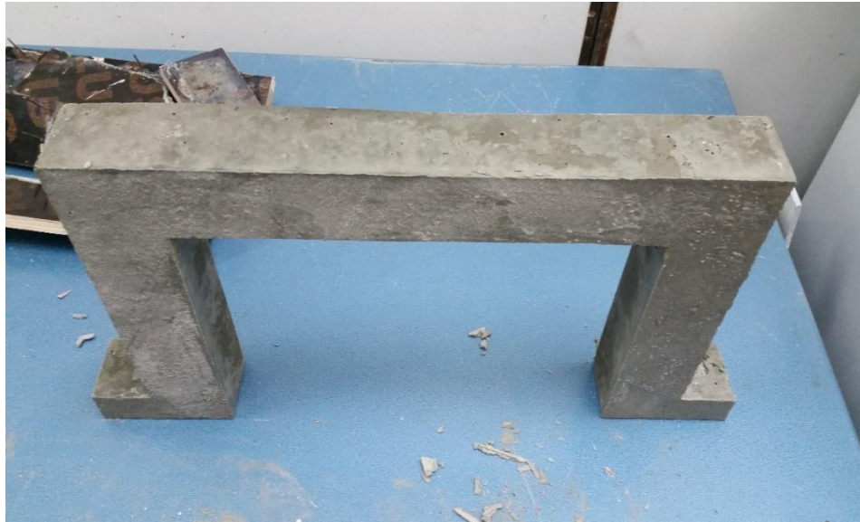
Figure 3.1 The investigated RC frame.
