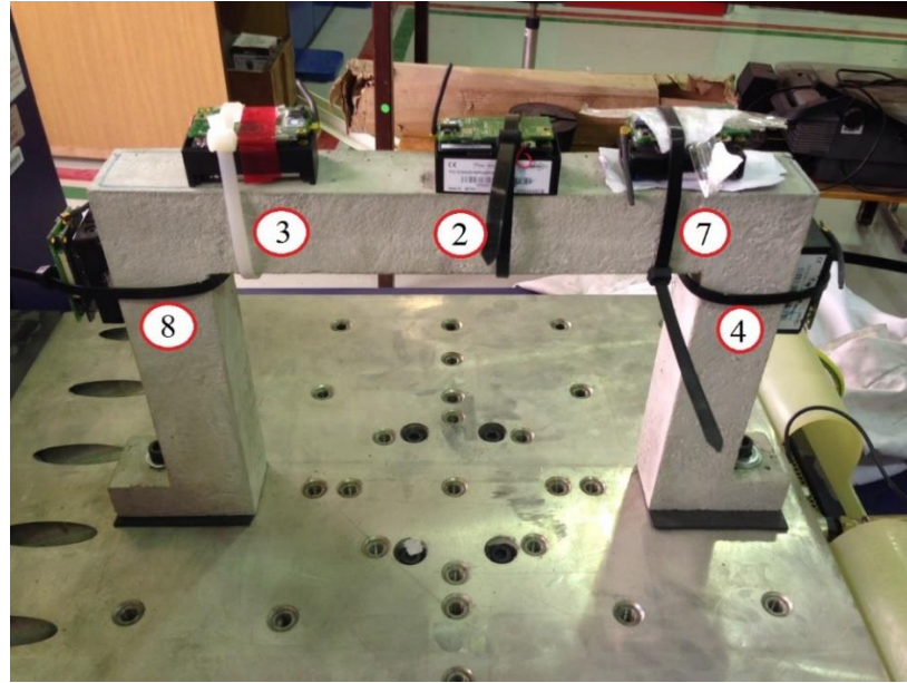
Figure 3.4 Wireless sensors arrangement mounted on RC frame.
