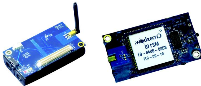
Figure 3.6 IRIS mote board top and bottom view.
