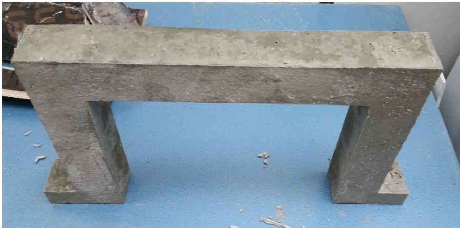
Figure 2.1 The investigated RC Frame.
