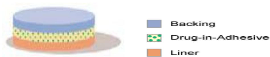
Figure 4.2 Diagram of a typical commercial nicotine patch [20]
