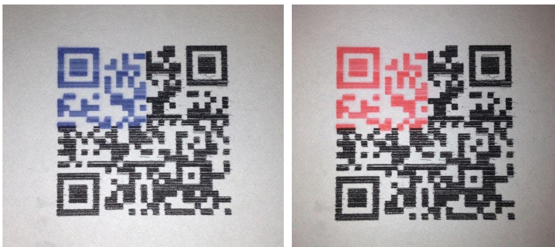
Figure 3.13 QR code with partial area of poly-TCDA/ZnO fabricated by inkjet printing methods.
