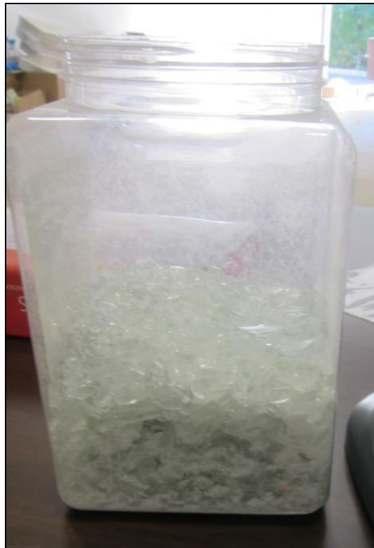
Figure A.3.18 Crushed Glass Used for Bioreactor
