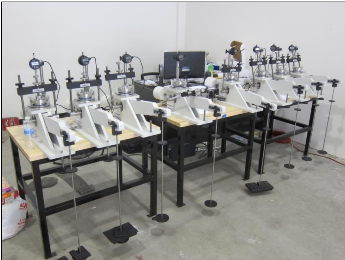
Figure A.3.1 Assembled Consolidation Machines and Data Acquisition
