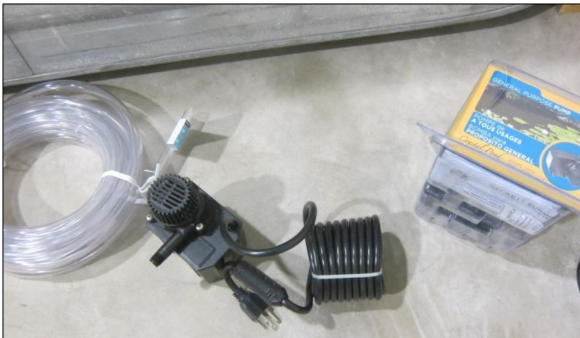
Figure A.3.8 Recirculation Pump for Water Bath
