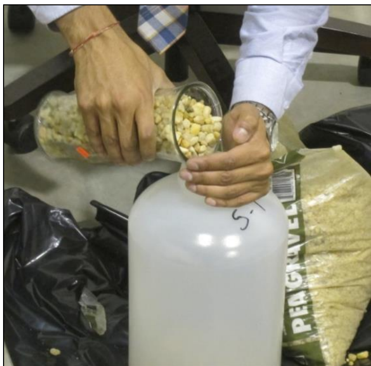
Figure A.3.27 Placement of Gravel Drainage Layer
