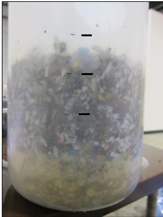
Figure A.3.30 Compacted Waste (note black marks used for lift thickness and measure density)
