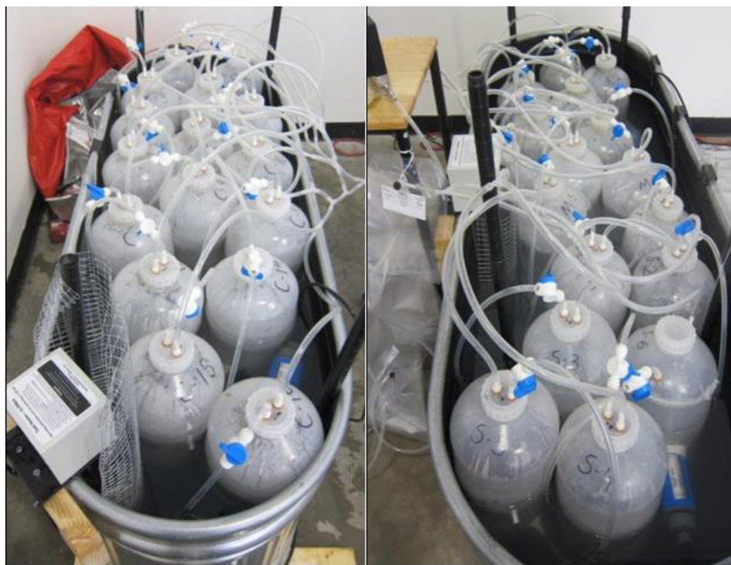
Figure A.3.31 Reactor Tank Assembled (Composite- Right, Individual – Left)
