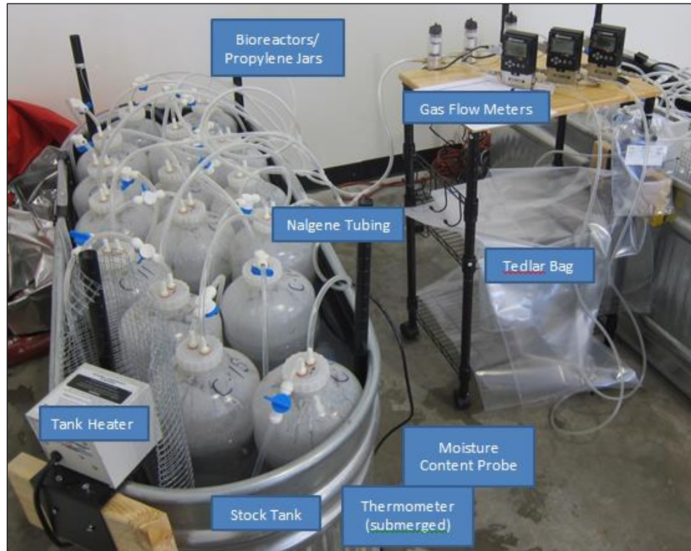
Figure 4.4 Bioreactor Test Set Up (Composite reactor tank shown)
