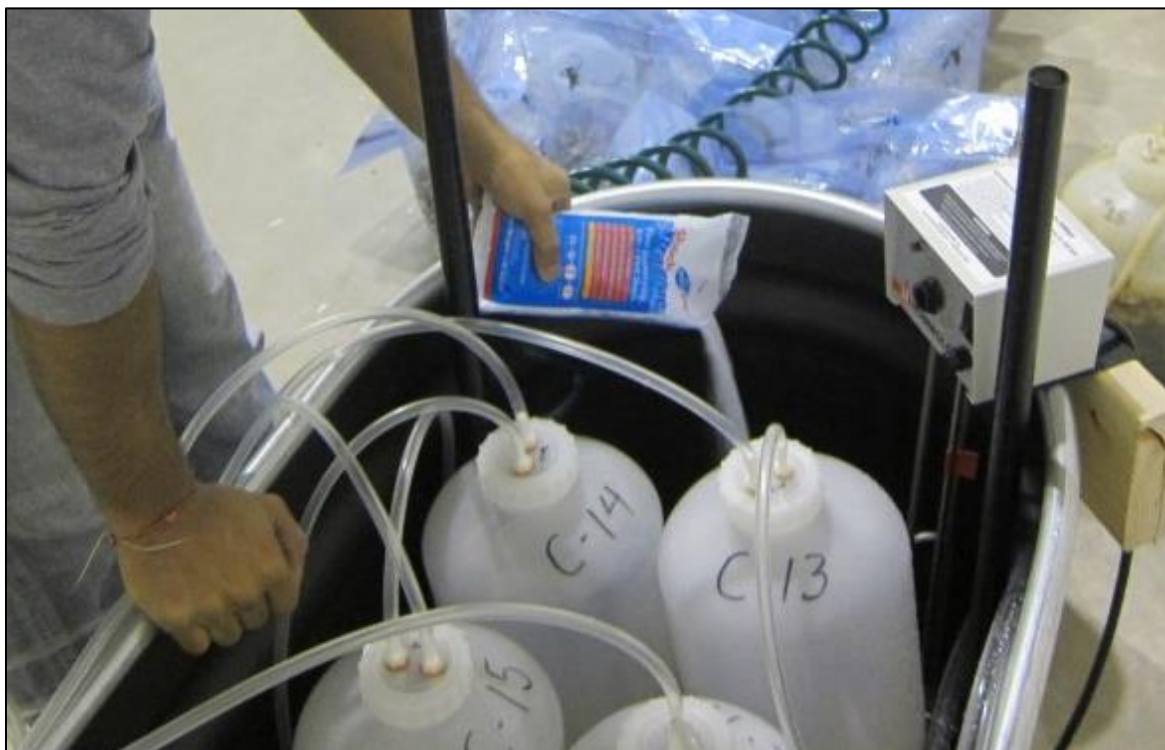
Figure A.3.9 Application of Anti-algae, anti-foam powder to water bath
