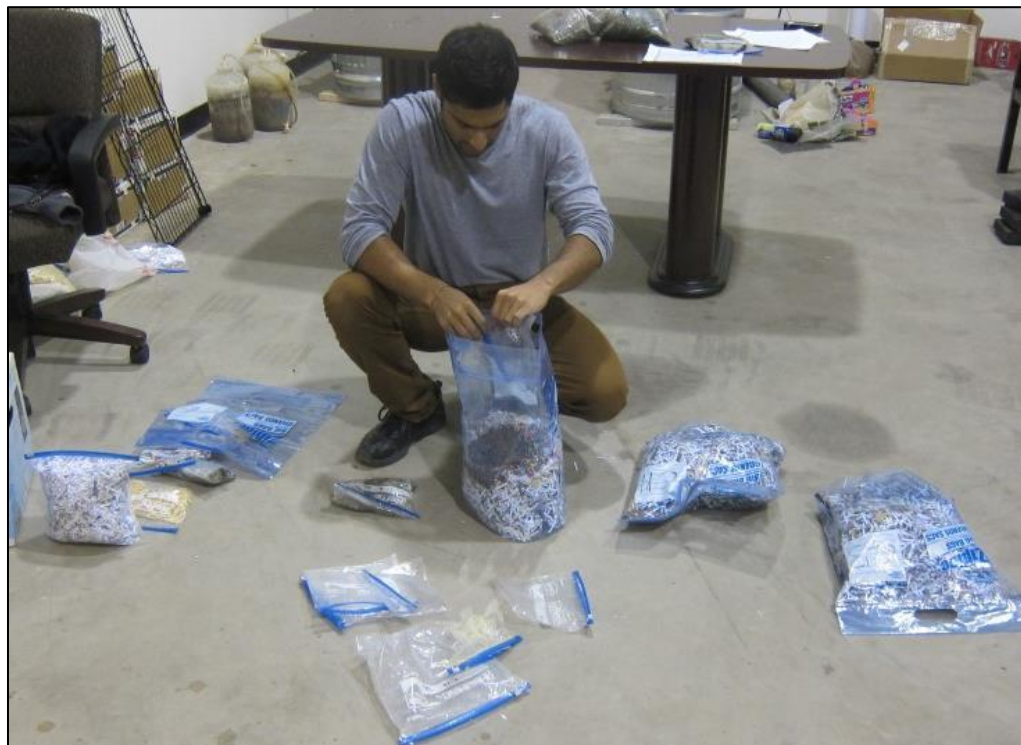
Figure A.3.25 Mixing Components to Create Bioreactor-specific Waste Mixture
