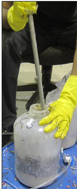
Figure A.3.29 Compaction of Waste into Bioreactor Using Tamping Rod
