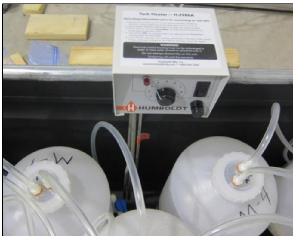
Figure A.3.3 Tank Heater for Water Bath
