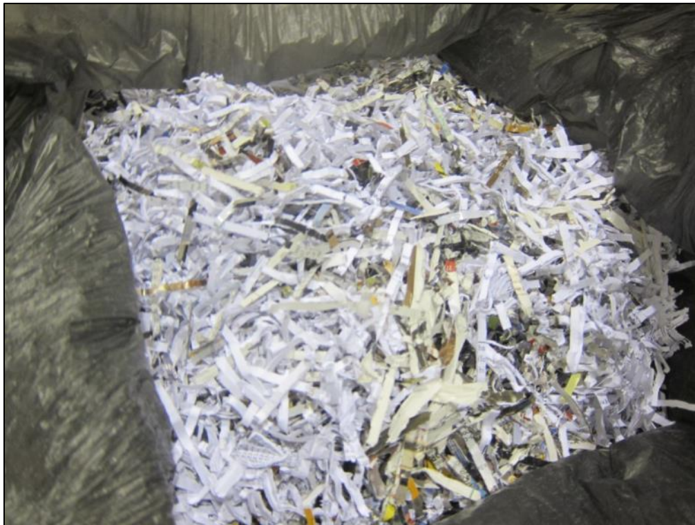
Figure A.3.14 Shredded Paper, Newspaper, Magazines, and Craft Paper Used for Bioreactors
