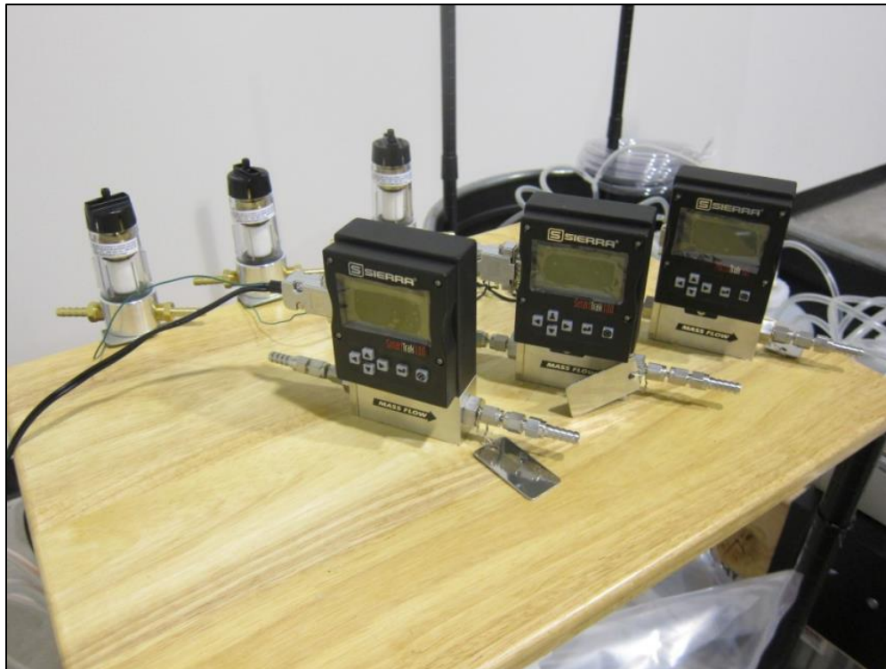
Figure A.3.6 Gas Totalizers for Methane Volume Determination
