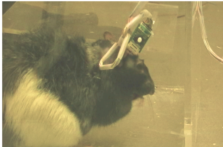
Figure 5.7 Picture of a chronically implanted rat while face cleaning, connected to a pre-amplifier via its skull- mounted percutaneous connector.
