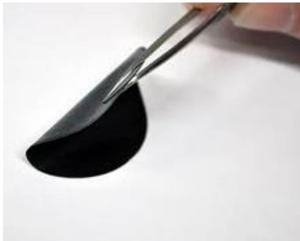
Figure 4.2 Carbon nanotube nanoper obtained after the sonication- filtration procedure.
