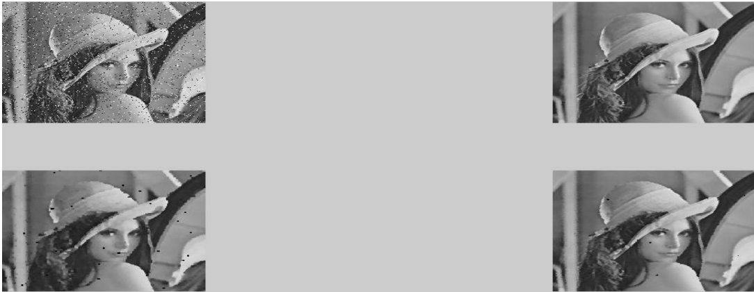
Figure 4.9 Salt and Pepper added to the Lena image (top-left), Morphological Smoothing with SE (disk type, radius 1) (bottom left); Morphological Smoothing with SE(2) (top-right); Morphological Smoothing with SE (disk type, radius 1) and SE (disk type, radius 3) (bottom-right).
