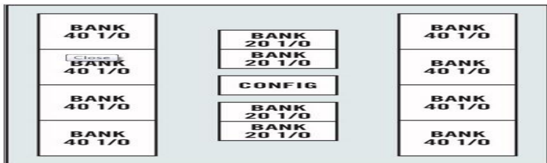
Figure 2.6 On-chip memory arranged in memory banks and available as BRAMs on Xilinx FPGAs.
