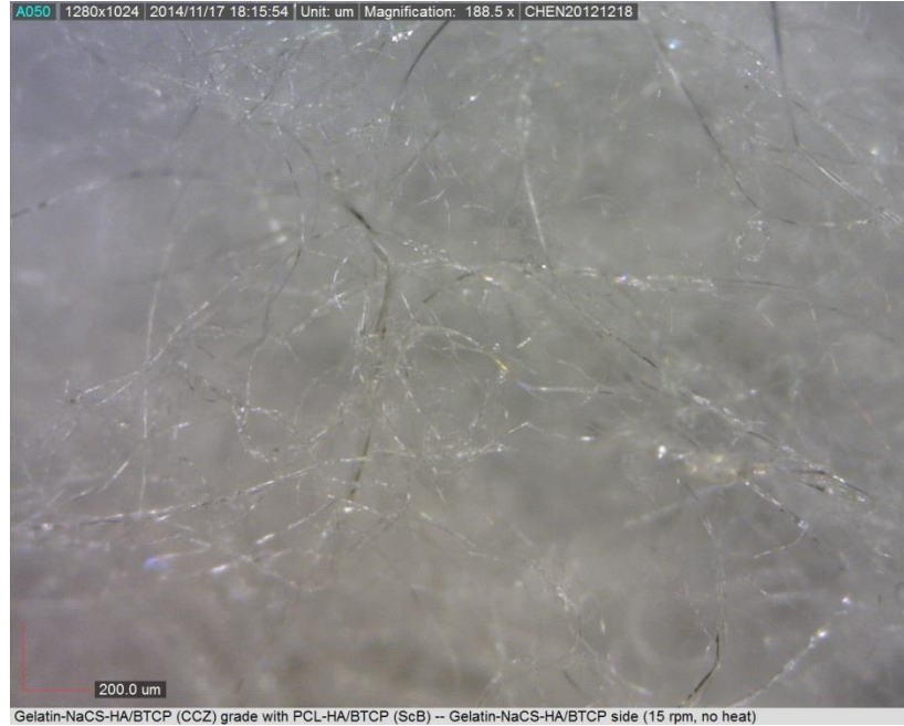
Figure 3.8 Light microscope image of the Gelatin-NaCS-HA/ \beta -TCP side of the Gelatin-NaCS-HA/ \beta -TCP//PCL-HA/ \beta -TCP scaffold.
