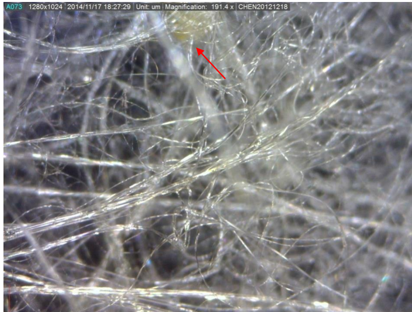
Figure 3.12 Light microscope image of the Gelatin-NaCS-HA/ \beta -TCP side of the Gelatin-NaCS//Gelatin-NaCS-HA/ \beta -TCP scaffold after heating 5 hours at 150°C. Gelatin aggregate is visible.
