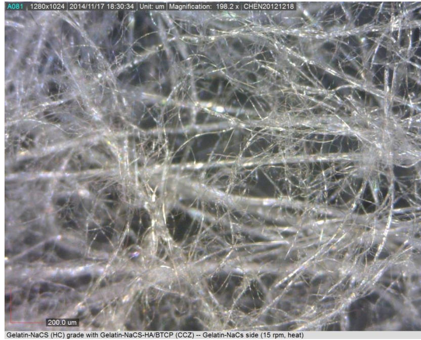
Figure 3.13 Light microscope image of the Gelatin-NaCS side of the Gelatin-NaCS//Gelatin-NaCS-HA/ \beta -TCP scaffold after heating 5 hours at 150°C.
