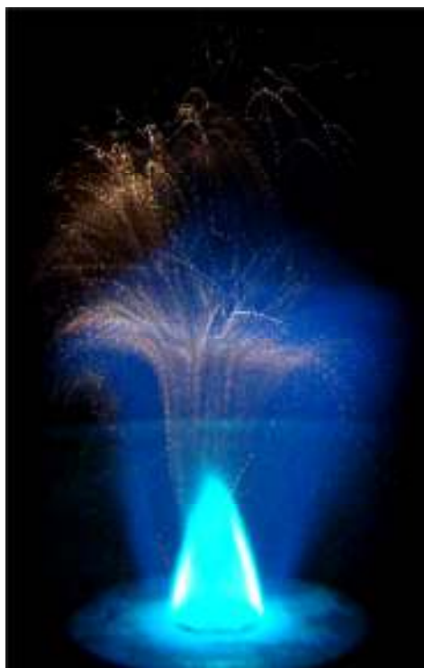
Figure 1.5. A characteristic side view image of a flame with burning Al particle streaks. The flow rates are: acetylene: 0.9 SCFH (standard cubic feet per hour), air: 10 SCFH, nitrogen: 2 SCFH. Turbulizing air flow is set at 100 SCFH.
