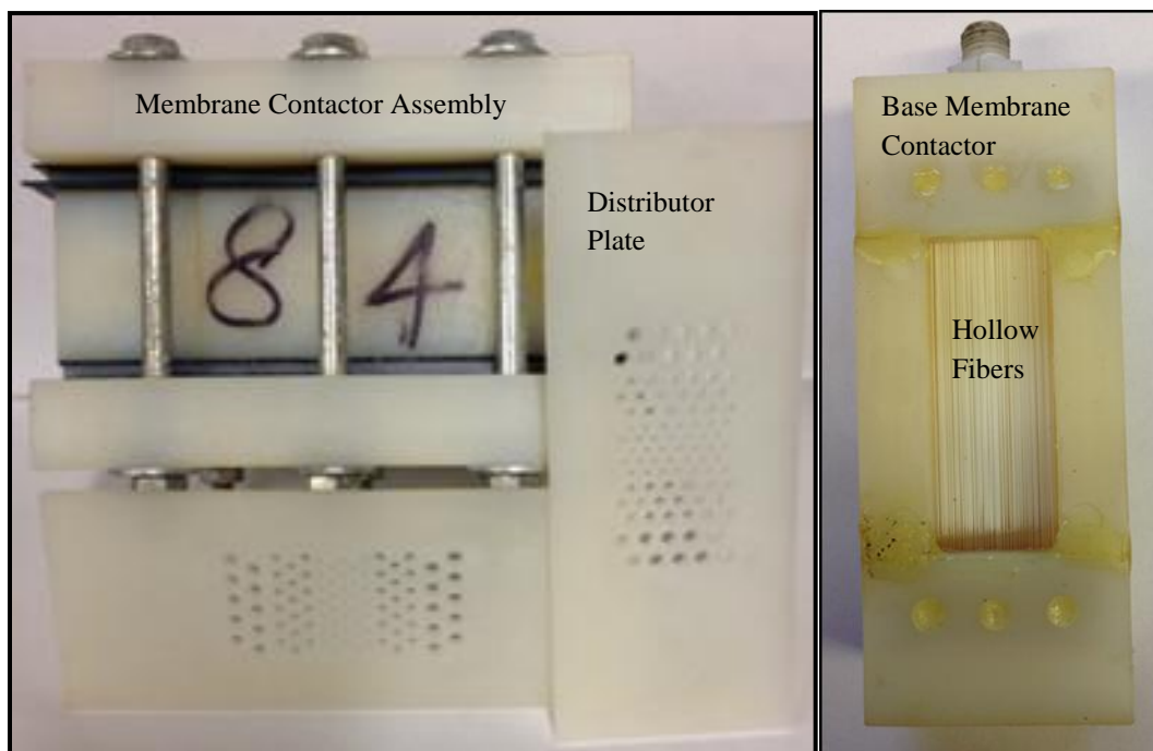
Figure 2.1 Rectangular assembly of cross flow hollow fiber membrane module contactor with face box and distribution plates.
