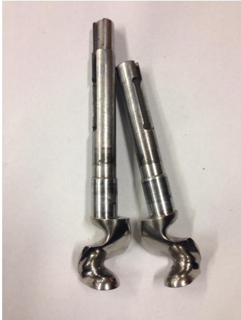
Figure 4.7 The intermeshing screw elements.
