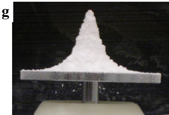
Figure 4.1 The results of the tests of the angle of repose: (a) \text{CaCO}_3 No.1, (b) \text{CaCO}_3 No.2 , (c) \text{CaCO}_3 No.3, (d) \text{CaCO}_3 No.4, (e) Soluplus (f) Aluminum (g) Acetaminophen (APAP)
