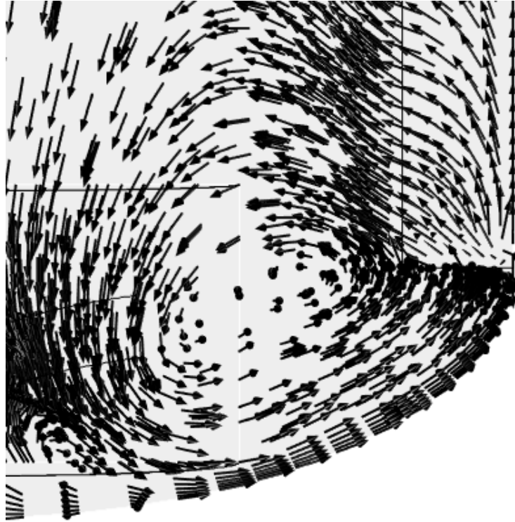
Figure 4.4 Close up of the velocity profile around the impeller, fully baffled system, 100 RPM, normalized vector flow field across each element, cross sectional slice of the yz plane down the center of the vessel.
