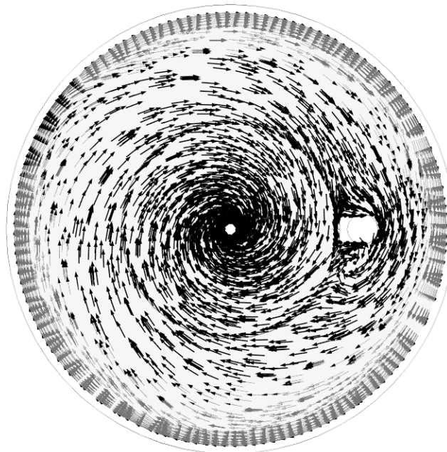
Figure 4.6 Top view of the velocity profile, semi-baffled system, 100 RPM, normalized vector flow field across each element, cross sectional slice of the xy-plane 100 mm from the liquid surface.
