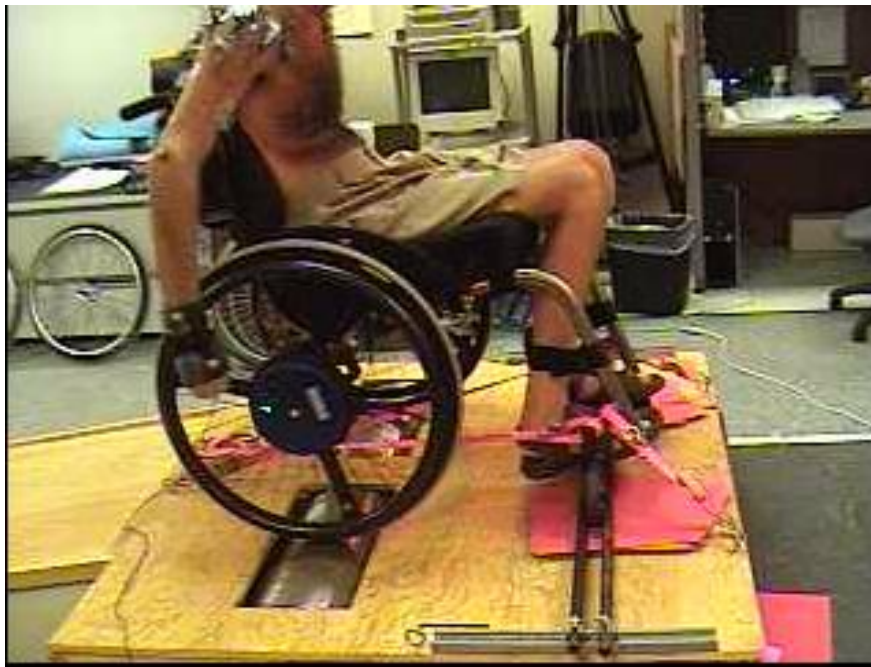
Figure 4.2 Experimental set up of the wheelchair propulsion study. Reflective markers were placed on the upper limb and trunk to track their position during the stroke cycle. Fine-wire electrodes were used to collect the muscle activity during the stroke cycle. Smart WHEELS were placed bilaterally on the wheelchair to record the force exerted by the hand to push rim during propulsion. The participant propelled his own wheelchair on a dynamometer that consisted of two independent steel tubular rollers (one for each wheel) using a four-belt tie-down system (Yarossi et al., 2010). Real-time speed feedback was presented on a monitor in front of the roller system.
